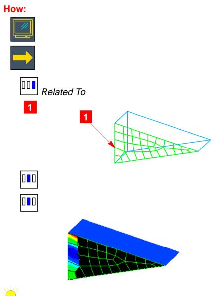
You can use this function to pick all elements or nodes on a surface to apply boundary conditions.
