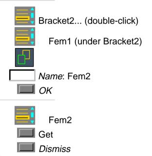
By making a copy rather than creating a new FE model, you save the steps of creating boundary conditions and re-meshing. The copy also contains any solved results.
