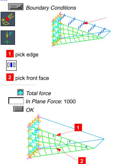
What: Verify that a boundary condition set still exists, containing the restraint and load.
